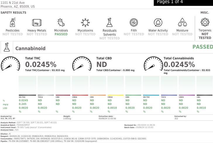
Full spectrum cannabinoid analysis utilizing High Performance Liquid Chromatography with Photo Diode Array detector (HPLC-PDA) for analysis. (Methods: SOP.T.30.500 for sample homogenization, SOP.T.30.031 for sample prep, SOP.T.40.031 for analysis on Shimadzu LC-20X0 series HPLCs). Potency results for cannabis flower products are reported on an "as received" basis, without moisture correction.
